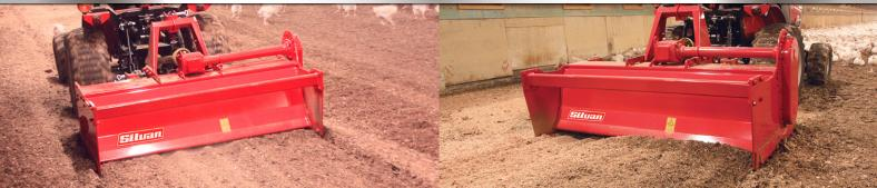
Following the introduction of new animal welfare regulations relating to the poultry industry, Silvan have specifically developed the Silvan Poultry Litter Rejuvenator (PLR) Rotary Hoe.
