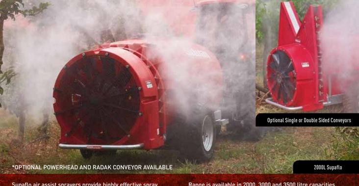
Supaflo air assist sprayers provide highly effective spray coverage in a wide range of crops such as grapes, apple, citrus, bananas, peaches and subtropical tree crops. Thanks to their proven features including the 900mm axial flow fan with air straightening vanes and high pressure diaphragm pumps, these sprayers deliver consistent and reliable spraying.
