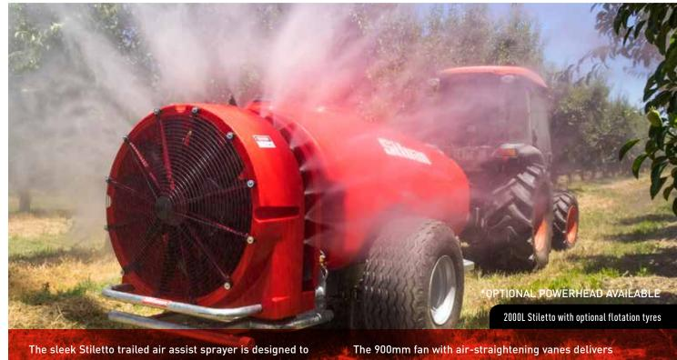
fit in the tightest orchard and vineyard rows with minimal disturbance to the crop. It incorporates a tough, low-profile 2000 litre poly tank which reduces the risk of snagging fruit on low branches, and a 15 litre built-in hand rinse tank for easy washing up.
