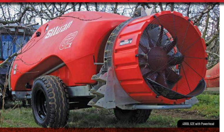
The Silvan 4000L G2E is a high capacity orchard sprayer in an economical package. It features Silvan's proven brass diaphragm pump and Glideflex suspension axle for a smooth ride. The G2E is available with either the Powerhead conveyor for medium size trees such as stonefruit, almonds and citrus or the Radak conveyor for tall trees.
