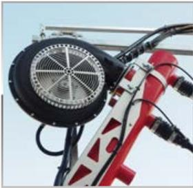
High performance hydraulic drive centrifugal fans are engineered to provide the high air velocity for optimum spray coverage.
