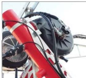
Fan hydraulic motor is isolated from the airstream meaning no chance of oil contamination if seals are compromised
