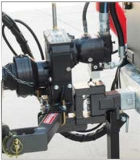
Hitch mounted hydraulic powerpack means PTO is protected and maneuverability is increased
