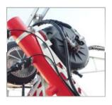
Fan hydraulic motor is isolated from the airstream meaning no chance of oil contamination if seals are compromised
