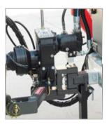
Hitch mounted hydraulic powerpack means PTO is protected and maneauverability is increased
