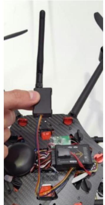
**Note:** The front of the UAV is the position for the camera which is also where the receiving antenna is located for the normal controller. Preferentially you should place the Telemetry transmitter/receiver away from the other transmitters/ receivers.
