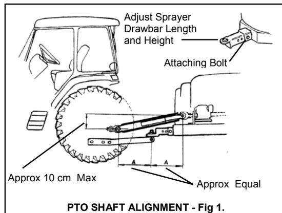
The hitch point between the tractor and sprayer should be approximately midway between the universal joints of the PTO shaft and the height difference between the joints should not be greater than about 10 cm, refer Fig 1. This will ensure the joint angles are approximately equal during turns and do not exceed the allowable limit.
