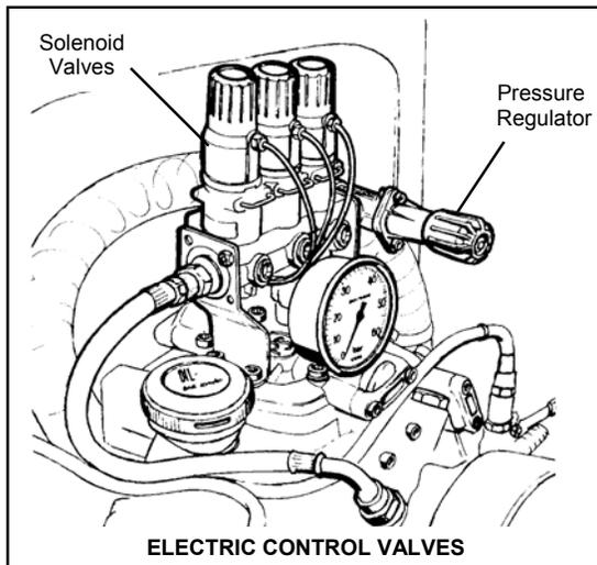
Spraying pressure is adjusted manually with the rotary control knob on the valve bank in the same way as the cable control system.
