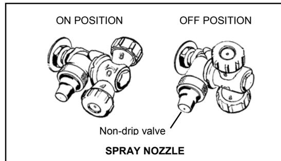
Nozzle direction can be adjusted +/- 15°. By loosening the attaching nut and angling the nozzle, greater adjustments can be made.
