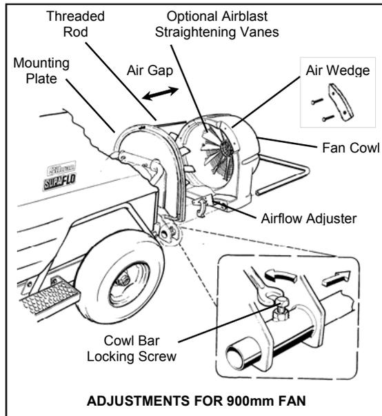
To adjust the gap, loosen the two grub screws on the underside of the cowl which clamp onto the slide bar at each side using a 5mm allen key. Loosen the nuts on the top threaded rod and move the cowl to the desired position. The minimum gap is 100mm and the maximum is 140mm. After adjusting, securely tighten the upper nuts and the lower locking screws.
