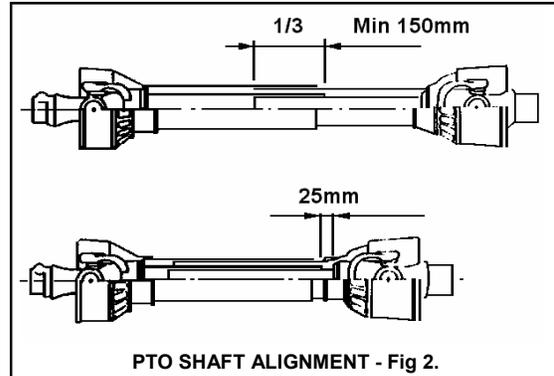
The telescoping tubes must overlap by at least 1/3 their length, but not less than 150mm, in all possible operating positions and there must be at least 25mm telescopic movement remaining at the minimum operating length, refer Fig 2.
