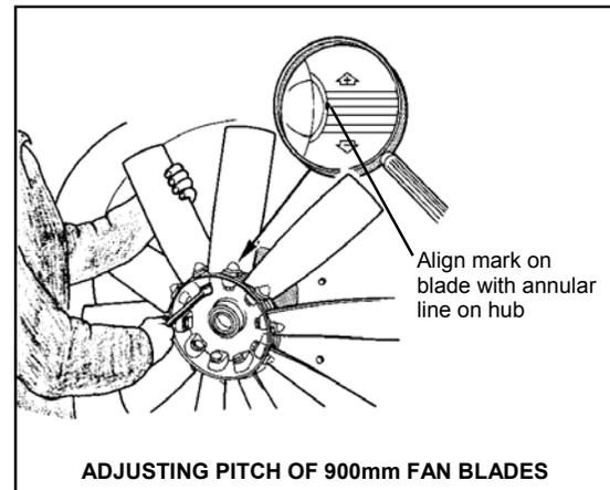
Normally when there is sufficient tractor power the fan should be operated at full pitch and if a lower volume of air is required the fan gearbox should be set in the low speed position.
