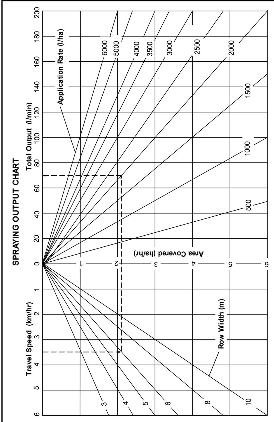
To use the chart draw a vertical line down from the Travel Speed axis, at the speed you will be using for spraying, until it intersects the diagonal line for the Row Width of your crop. From this point draw a horizontal line to intersect the diagonal line for the Application Rate that you have chosen, then draw a vertical line up to the Total Output axis to show the total litres/min you will need to use.
