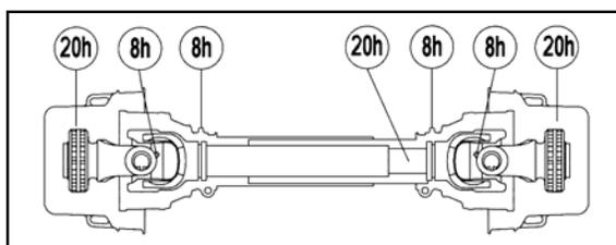
Every 20 hours slide the PTO shaft apart, clean the telescopic tubes with kerosene and apply multi-purpose grease to the sliding surfaces, then reassemble. This is most important in dusty conditions.
