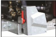
The manual pressure regulator on the discharge side of the pump is used to set the system maximum pressure, which is set higher than that required for spraying to ensure correct operation of the electric pressure regulator. Excess fluid from the pump is by-passed through the manual regulator back to the tank and helps keep the contents agitated.
